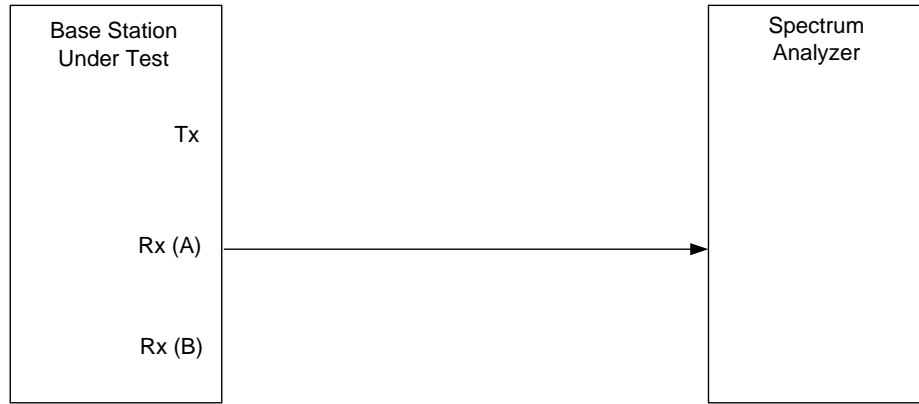
Figure 22 - Test setup: conducted spurious emissions
